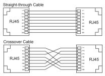
Figure 11 Connection Using Straight-through/Cross-over Cable
