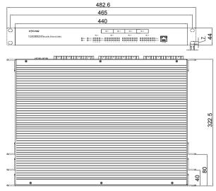
Figure 3 Dimension Drawing (unit: mm)
