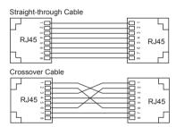
Figure 8 Connection Using Straight-through/Cross-over Cable
