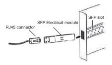
Figure 16 Connecting the Gigabit SFP Electrical Module
