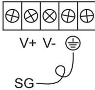
The Shielded Ground (sometimes called Protected Ground) contact is the second contact from the right of the 5-pin power terminal block connector located on the rear panel of NPort 5600 VDC. Connect the SG wire to the Earth ground.
